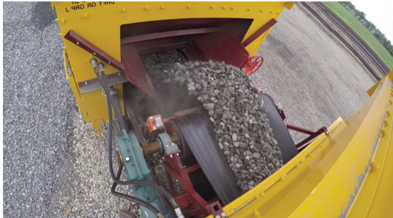
Shown: Herzog Railroad Services Inc.'s Automated Conveyor Train unloading material in a curve.
